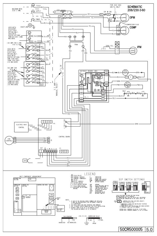
Fig. 16 - Wiring Schematics-50CR Three Phase
